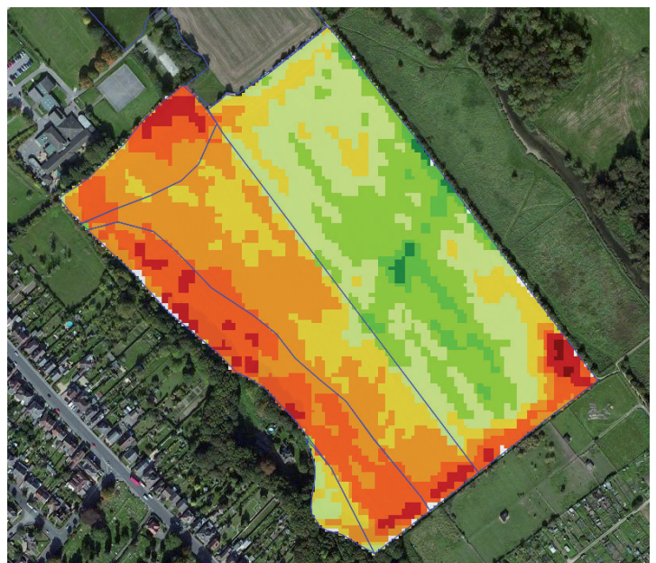
NDVI image showing how crop biomass imagery matches the soil management zones.
