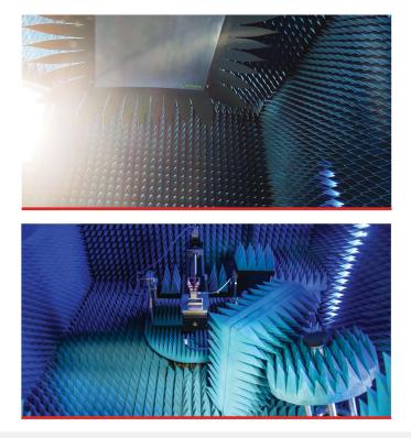
The Compact Antenna Test Range facility is particularly suitable for the dynamic over-the-air performance testing of electronically steerable antennas and terminals for Satcoms or 5G applications in the frequency range 10GHz to 31GHz, offering a quiet zone upto 42cm. The Compact Range is available for daily or monthly lease (subject to availability) and our experts are on hand to support you with each stage of your product's testing and development.
