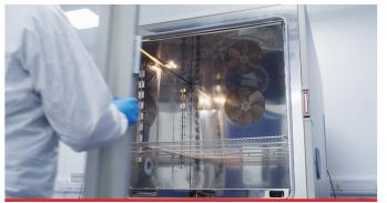
The Environmental Chamber provides atmospheric and temperature testing for your aerospace equipment with a 1076 litre capacity and a temperature range from -75°C to 180°C. The Environmental Chamber is available for short, medium, or long-term use (subject to availability) and our experts are on hand to support you with each stage of your product's testing and development.
