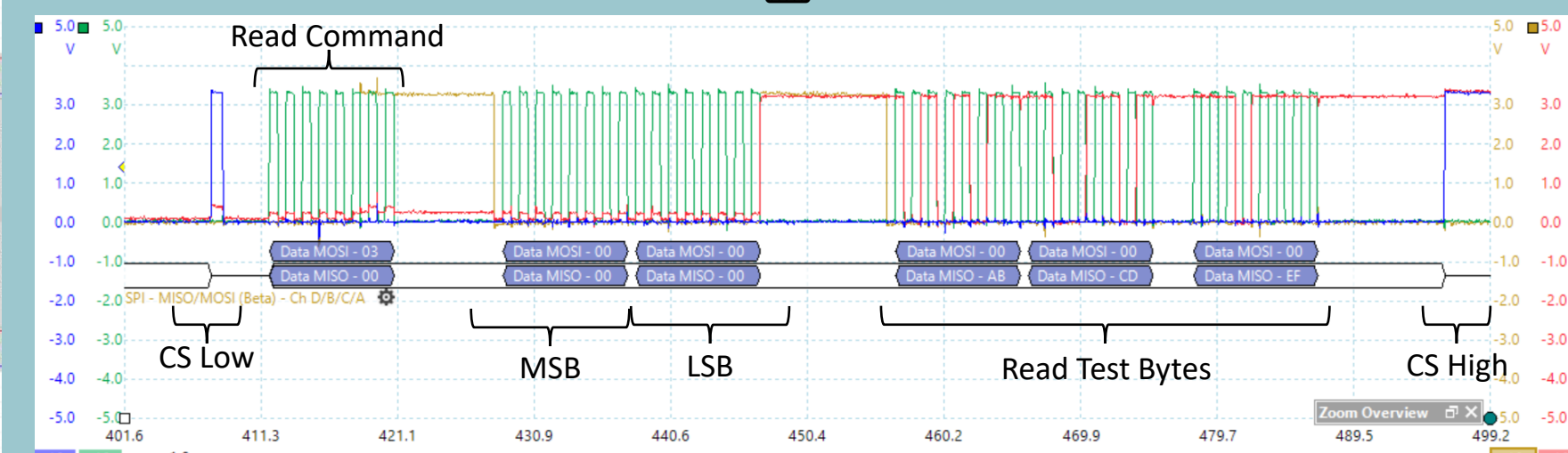
Figure 7: Waveform of a read cycle to the SRAM
