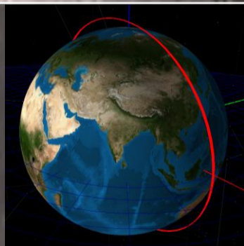
Figure 2: GMAT simulation of a satellite in a polar SSO at 600 km (red)
