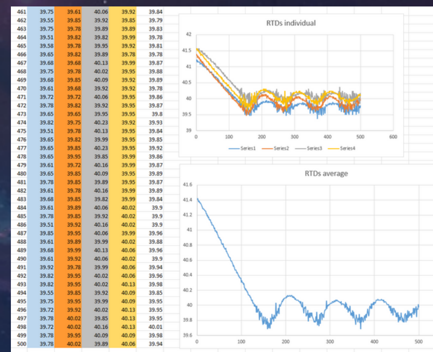
Figure 3 Variation of temperature with time of a mirror heated to 40°C
