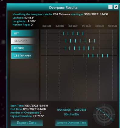
Fig.5 The screenshot taken from the MagTrack software. Shows the overpass calculation interface, with overpasses calculated for few satellites at ESA Cebreros station.
