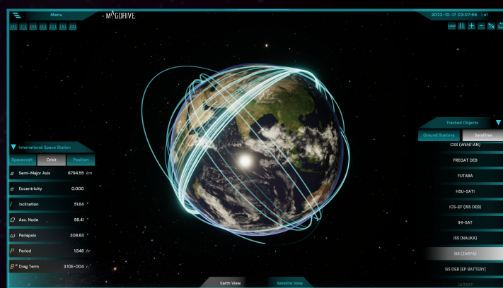
Fig.2 The screenshot taken from the MagTrack software, shows Earth along with several of visualized orbits. The user interface on the right shows the list of currently tracked objects.
