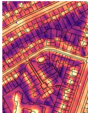
Figure 2: Snapshot of QGIS map with OS polygons (black lines) showing buildings and roads on top of Satellite Vu brightness temperature data. Each polygon has a unique feature ID. [3]
