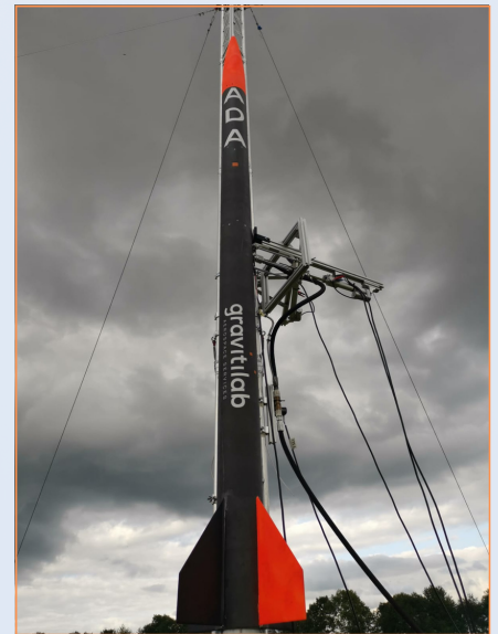
Launch vehicle positioned on the launch structure and connected to the umbilical ground system ready to be pressurized prior to launch.
