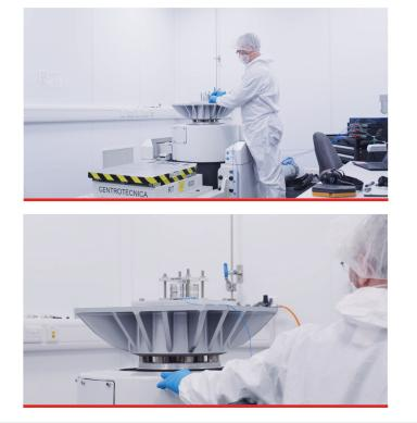
Our Vibration Table allows fast and accurate vibration testing of satellites and components. Operating at a peak force of 22kN, it is ideal for Cube Sats and other small satellites. Quick transformation between horizontal and vertical axis means no delays in testing.
